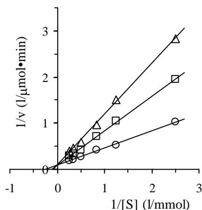
**Figure 2.** Lineweaver-Burk plot for the competitive inhibition of metyrapone reduction by androsterone and cholic acid. The carbonyl reductase activity of  $3\alpha$ -HSD was assayed for the metyrapone concentration range from 0.4 mM to 4.0 mM in the absence (circle) or presence of 0.1 mM inhibitor, androsterone (square) and cholic acid (triangle).
