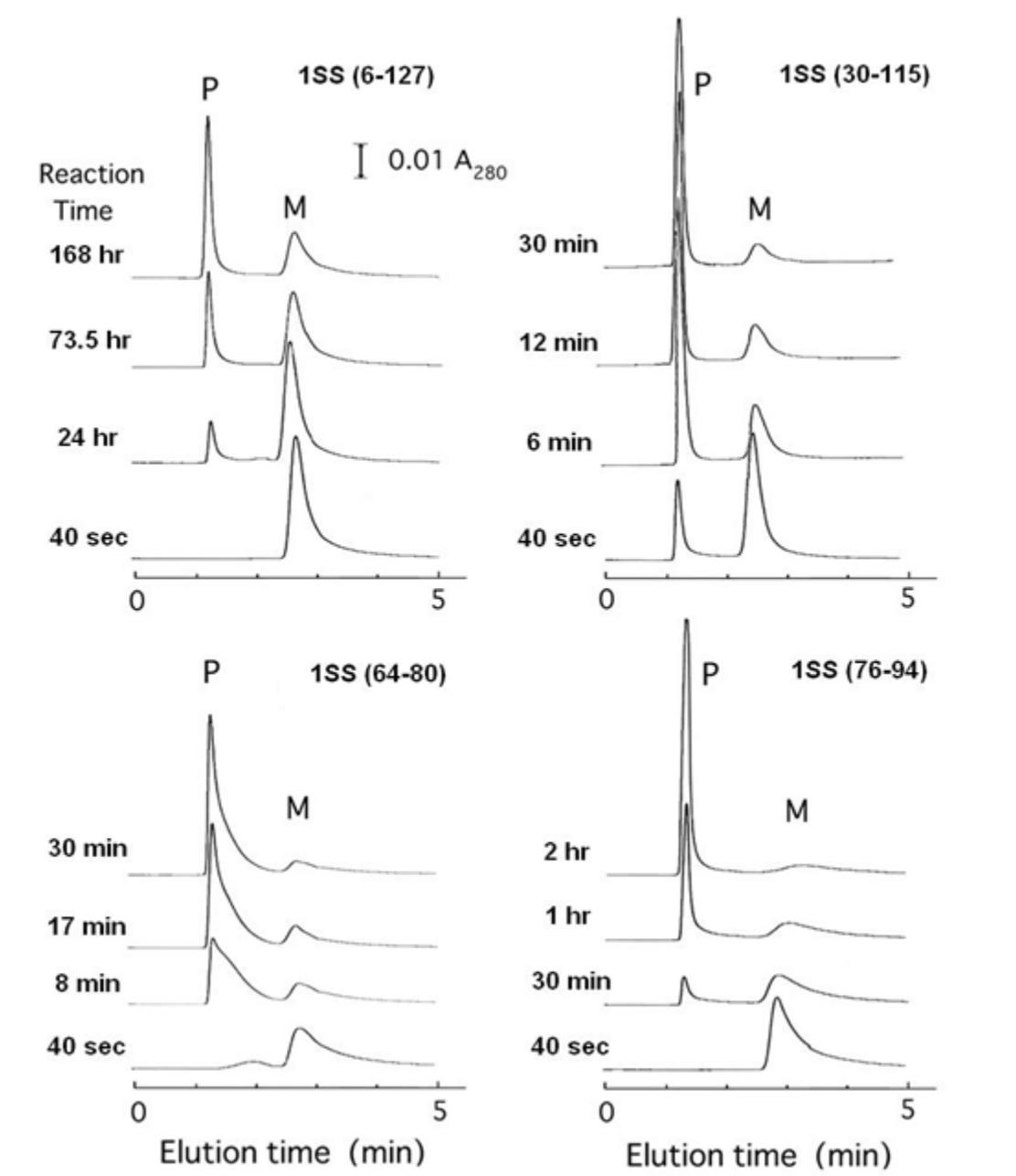
**Fig. 3.** Changes in SEC elution profiles of the 1SS variants with the progress of fibrillation. Each 1SS solution,  $4 \text{ mg ml}^{-1}$  in  $20 \text{ mM}$  sodium acetate,  $\text{pH } 4.0$ ,  $50 \text{ mM}$   $\text{NaCl}$ , was incubated at  $25 \text{ }^\circ\text{C}$ . At each incubation period labeled to each profile aliquot of the solution containing  $10 \text{ } \mu\text{g}$  protein was subjected to SEC. P and M denote polymer and monomer peaks, respectively.
