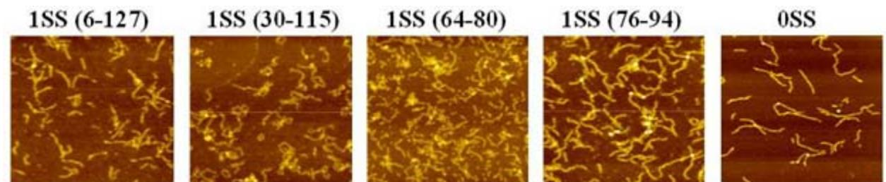
**Fig. 2.** AFM images of the fibrils of the 1SS-variants and 0SS. Fibrils were formed by incubating 5 mg ml<sup>-1</sup> each variant protein in 20 mM sodium acetate, pH 4.0, 50 mM NaCl at 25 °C for four days (1SS (6-127)) or one day (1SS (30-115), 1SS (64-80), 1SS (76-94), and 0SS). All images are 1  $\mu$ m  $\times$  1  $\mu$ m in an observation window size.
