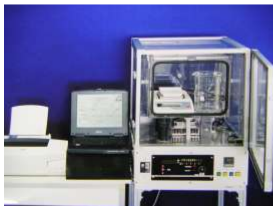
Fig.1 A photograph of the evaporation rate measuring device developed by Shin-ei Sangyo, Co. Ltd, Osaka, Japan.
