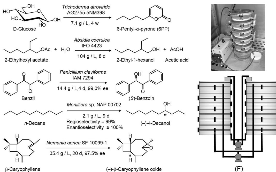
**Fig. 4. Application of L–L IBR to various fungal bioconversions and a photograph and a schematic diagram of a multi-story L–L IBR system. The system consisted of stacked reactor units, diaphragm-pump, and solvent-circulation lines to connect an organic phase.**
