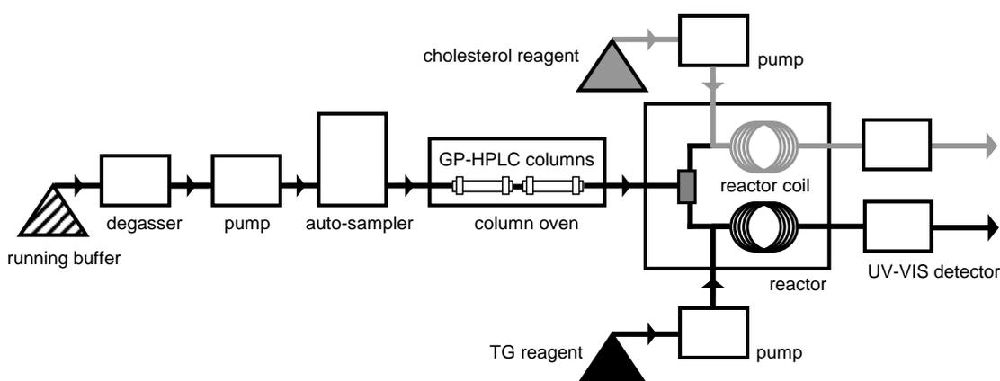
Fig. 2. Configuration System of LipoSEARCH®.
